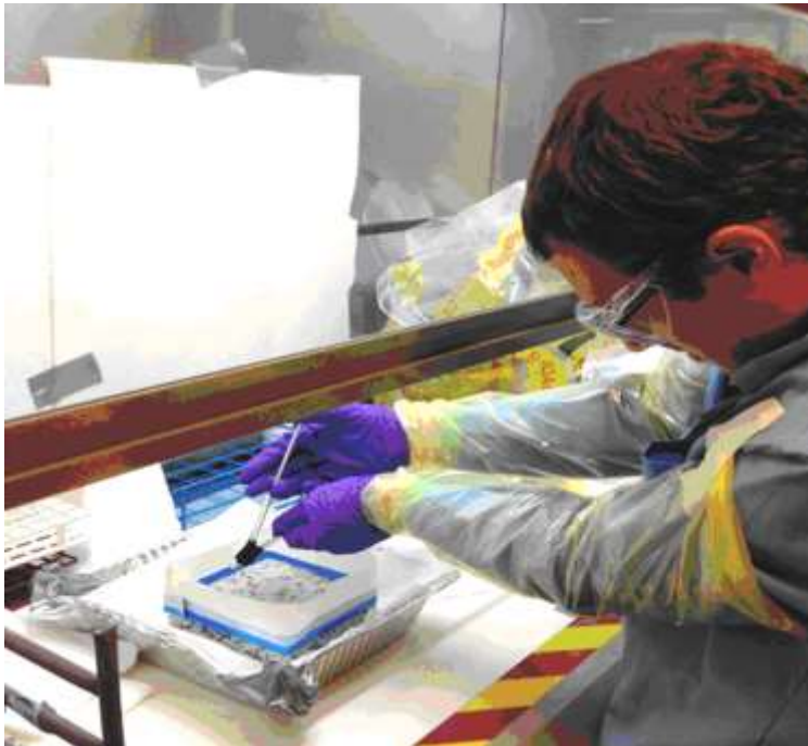
Figure 1. Spraying a building material coupon with a radioactive contaminant.
